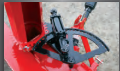
Gear-to-gear hydraulic chute rotation with cylinder
